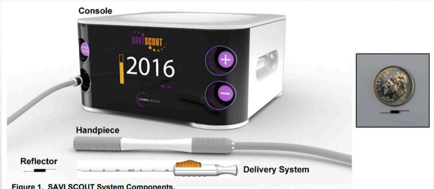
Figure 1. SAVI SCOUT System Components.
